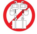
NEVER use 2 or more hoists to lift a load above capacity of a single hoist
