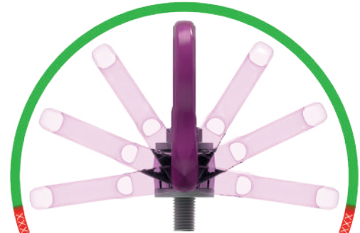
Pic. 10: Pivoting area (green = permitted loading direction)
