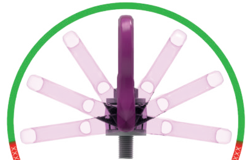
Pic. 10: Pivoting area (green = permitted loading direction)
