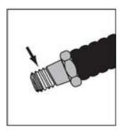
Connect the hose and cylinder couplers by hand, ensuring that they are fully engaged prior to use. Always connect hoses to both ports on a doubleacting cylinder, never attempt to pressurise a double-acting cylinder that only has one hose connected.
