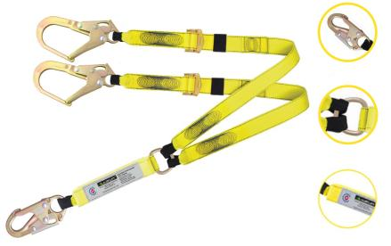
Double Action Snap Hook: made of forged alloy steel, MBS 23kN. Gate opening 20mm, with golden yellow galvanised finish. ANSIZ359.12-2009 - 16kN gate
