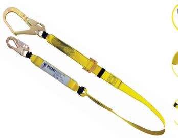
Double Action Snap Hook: made of forged alloy steel, MBS 23kN. Gate opening 20mm, with golden yellow galvanised finish. ANSIZ359.12-2009 - 16kN gate
