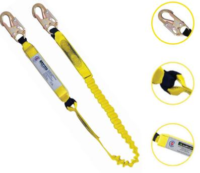
**Double Action Snap Hook:** made of forged alloy steel, MBS 23kN. Gate opening 20mm, with golden yellow galvanised finish. ANSIZ359.12-2009 - 16kN gate
