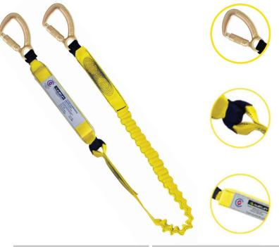
**Triple Action Locking Snap Hook:** made of forged alloy steel, MBS 23kN. Gate opening 19.5mm, with golden yellow galvanised finish.
