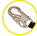
**Double Action Snap Hook:** made of forged alloy steel, MBS 23kN. Gate opening 20mm, with golden yellow galvanised finish. ANSI Z359.12-2009 - 16kN gate
