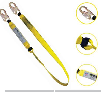
Double Action Snap Hook: made of forged alloy steel, MBS 23kN. Gate opening 20mm, with golden yellow galvanised finish. ANSIZ359.12-2009 - 16kN gate
