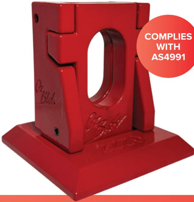
The **OzBlok Road Plate Lifter** system comprises of a receiver plate and a lifting tool. Once the receiver is flush welded at the centre of a steel trench plate, the lifting tool can be inserted into the receiver and locked into position before a hook is attached to the middle of the lifting tool. The flush welding reduces risk of tripping and allows for plates to be conveniently stacked.
