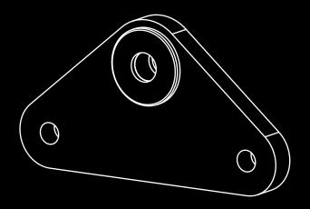
When using multiple sling legs this device provides a means of equalising forces within the legs. Connection is made via standard Grade "S" bow shackle and can be used with chain, wire rope or synthetic slings. Ideal in compensating for differences in load lift points and sling lengths.
