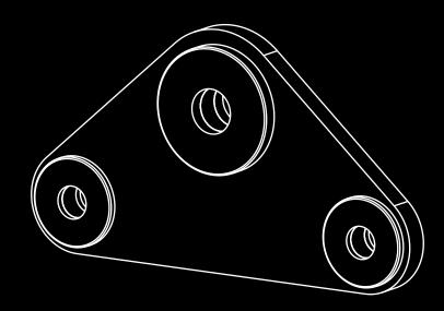
When using multiple sling legs this device provides a means of equalising forces within the legs. Connection is made via standard Grade "S" bow shackle and can be used with chain, wire rope or synthetic slings. Ideal in compensating for differences in load lift points and sling lengths.
