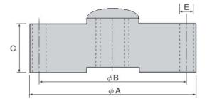
Wirop provides compression loadcells, Capacity ranges from 2.5T to 100T. The compression loadcell coupled with the Centre of Gravity solfware package. The centre of gravity can be easily found. The loadcell is made of high grade stainless steel making the loadcells are particularly suitable for rugged environments.
