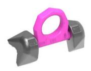
A forged ring bracket according to EN1677-1, electromagnetically crack detected, and it can be loaded in all directions. Even force distribution owing to the two point attachment. Low profile sice it can be folded with in an angle range of 270°. The welding block for edges is forged out of a good welding material 1.0577+N (St 52-3) and clearly stamped with an identification number for the permissible WLL. Welding should only be carried out by qualified persons according to ISO 9606-1.
