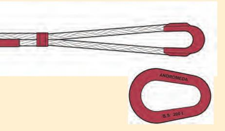
"A" thimble -designed to engage directly into clevis and pin on haul truck, will also accept alloy steel shackle of appropriate size
