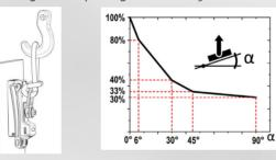
Maximum load weight with 3:1 safety factor =  $\underline{622 \text{ kg x } 100\% \text{ x } 30\% = 186 \text{ kg}}$ Maximum load weight with 3:1 safety factor =  $\underline{1365 \text{ lbs x } 100\% \text{ x } 30\% = 410 \text{ lbs}}$
