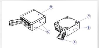
A) Activation leverB) Aluminium housingC) Threaded holes for attachmentD) Magnetic surface
